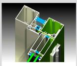
Will accept hinged, pivot or sliding doors. Doors are 50mm thick. Heavy duty adjustable hinges with extruded aluminium backing plates designed to support heavy door panels. The wide stiles allow us to fit wide backset locks.
